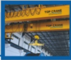
DOUBLE GIRDER EOT CRANE
