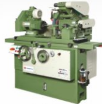
Cylindrical Grinding Machine 150 x 300 mm
