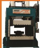
Deep Drawing Hydraulic Press ( 450 Ton )
